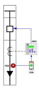
Figure: 4: Single point sensor - Cable box
