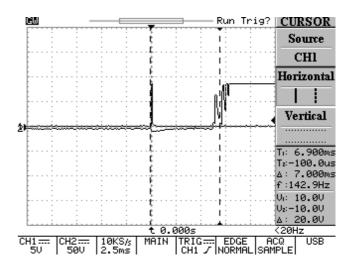
CRO trace showing nominal operation time of the trip contacts at 7ms. First contact touch at 6.25ms and fully closed by 7.25ms. Operation in <10ms is considered acceptable as current check relay operate time is ~15ms.
