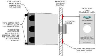
Figure 16: Panel mount version side view
