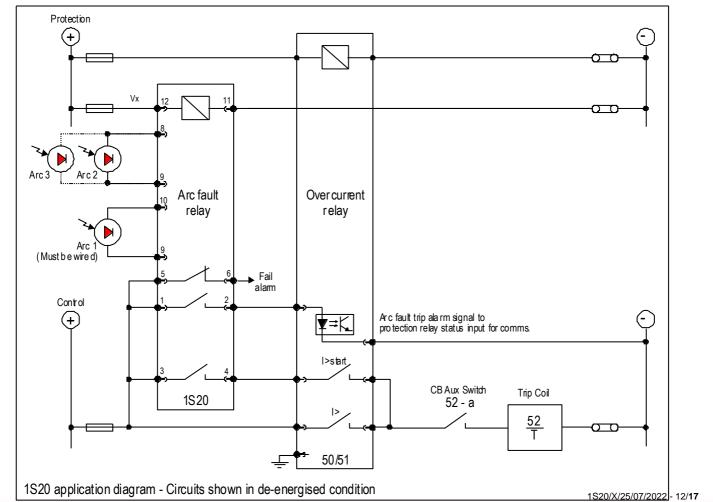
Note: \* Always wire Arc Sensor 1. Arc Sensors 2 & 3 are optional
