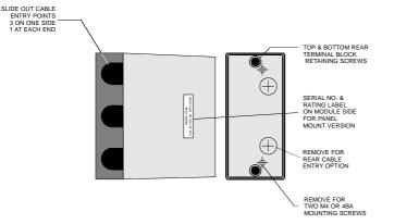
Figure 14: Surface mount version side view
