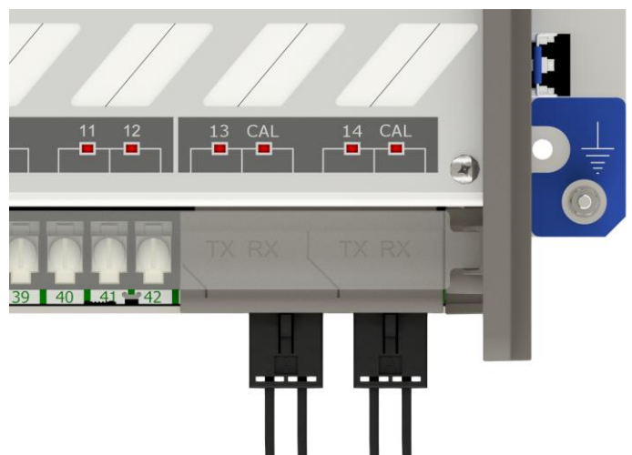
Figure 31: 1S40 Rx and Tx optic fibre connections
