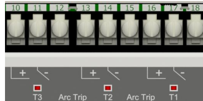
Figure 10: Arc trip output contacts and trip LED
