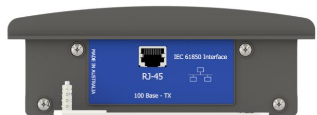
Figure 19: Standard single port 10Base-T / 100Base-TX
