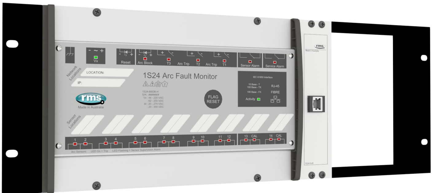
Figure 37: Rack mount version showing RJ45 socket fitted
