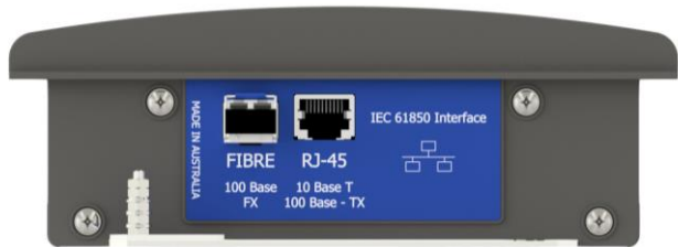
Figure 20: Optional dual port 10Base-T / 100Base-TX + 100Base-FX
