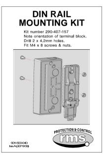
DIN rail clip fitting detail - Specify DIN Rail Mounting Kit P/N 290407157
