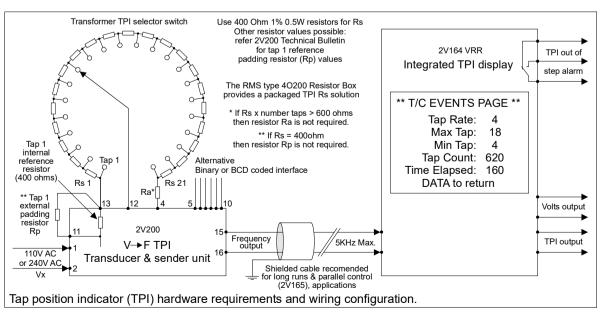
Figure 1 – Application diagram
