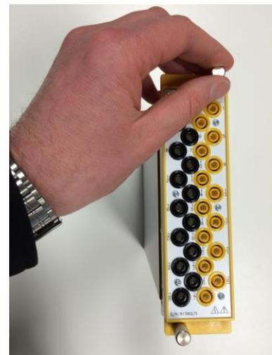
Test Plug inserted into test block, tighten thumb screws to retain in position
