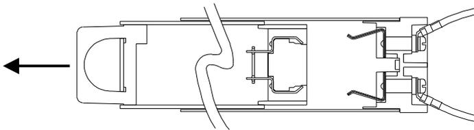
WITHDRAW DC AUXILIARY ISOLATION PLUG (4M300-B model only)
