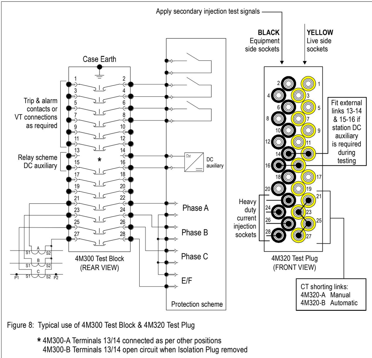
Figure 8: Typical use of 4M300 Test Block & 4M320 Test Plug
