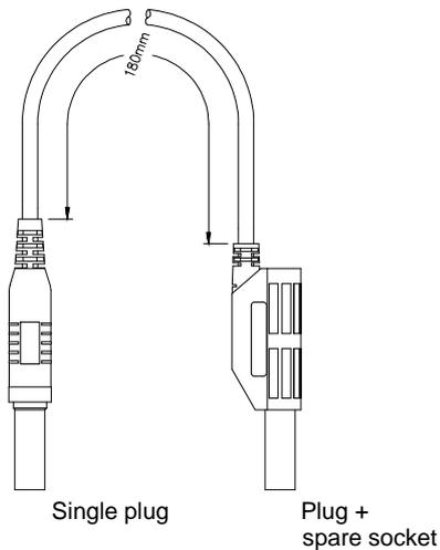
Figure 5: Two ended test lead - long
