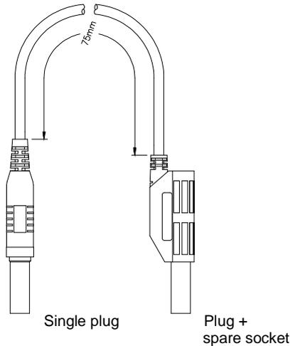
Figure 4: Two ended test lead - short
