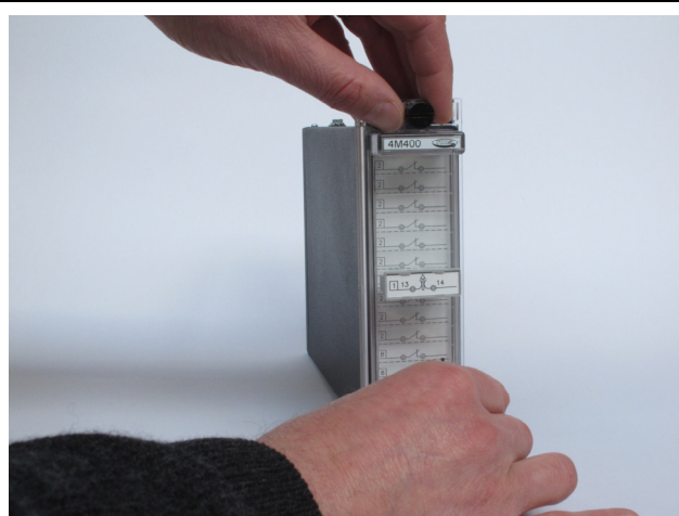
Undo Front Cover Thumbscrews to allow Front Cover Removal
