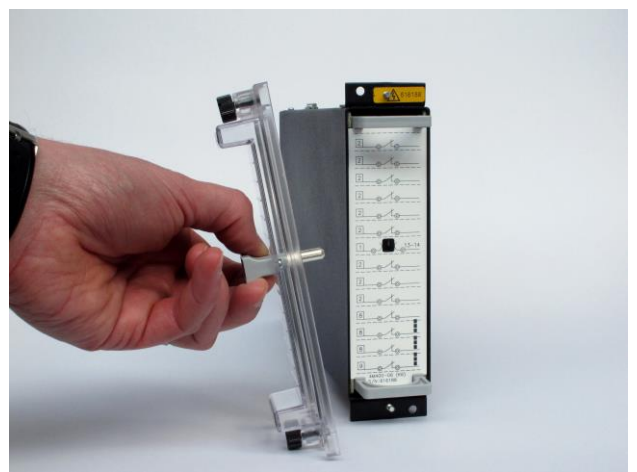
Front Cover Removed - Stage 1 Isolation Completed
