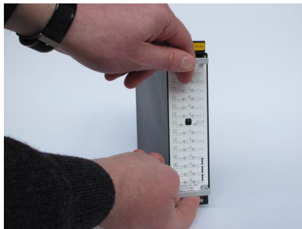
Withdraw Isolation Plug - to Automatically short CT circuits and then isolate remaining circuits
