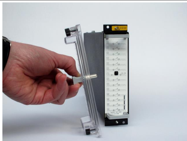
Test Block Cover restoration
