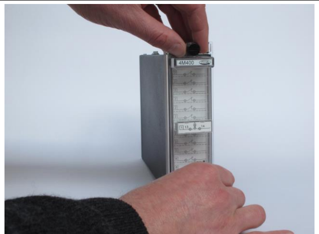
Tighten Test Block Cover screws
