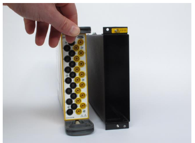
Test Plug extracted and test block ready for isolation plug insertion
