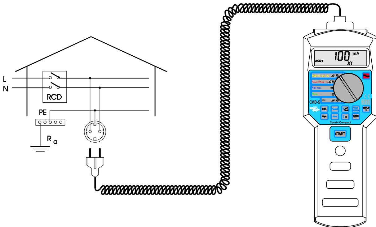
**Line ( $Z_{LINE}$ )- or loop ( $Z_{LOOP}$ ) impedance
