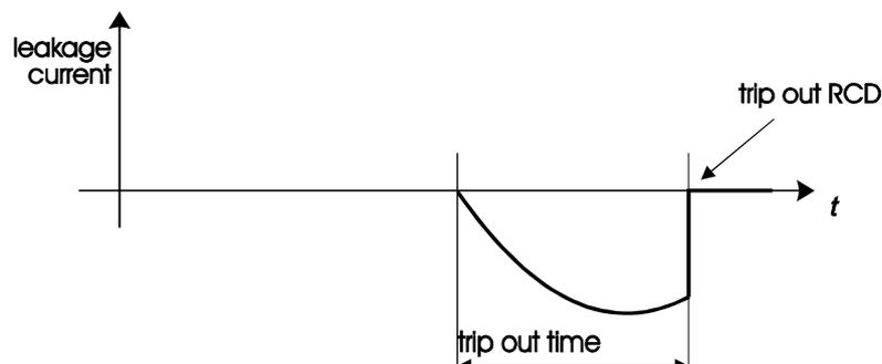
Figure 2: Alternating fault current.
