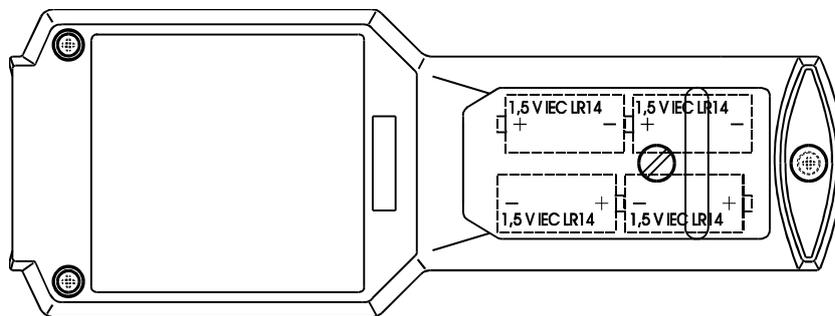
Figure 12: Batteries inserted
