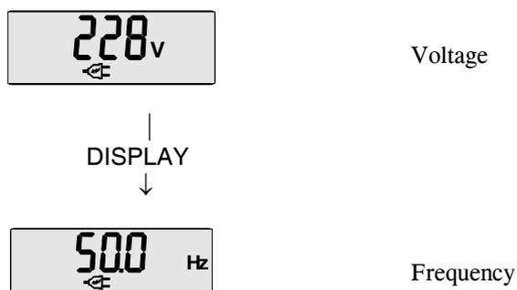
Figure 10: Example testresult mains voltage and - frequency
