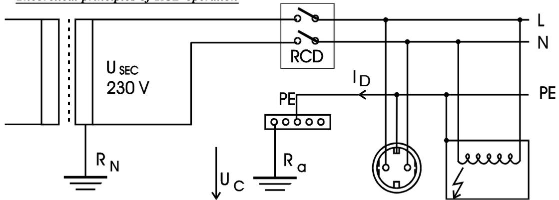
Figure 1: TT system connection
