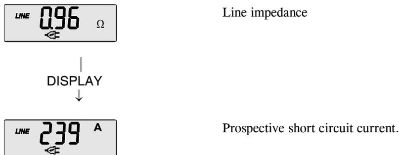
Figure 8: Example line impedance and prospective short-circuit current
