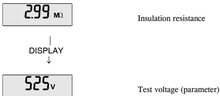
Figure 9: Example testresult insulation resistance and test voltage
