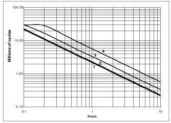
By connecting 2 contacts in series, the DC current breaking capacity is increased by 50%.
