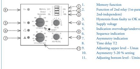
Function of 2nd relay (1st-paralel, Hysteresis from faulty to OK normal state Indication overvoltage/undervoltage, failure Sequence indication Asymmetry indication Adjusting upper level – Umax Asymmetry 5-20 % setting
