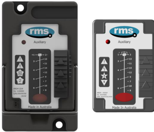
Figure: 1: ARD4 front panel Left – Panel mount Right – rail mount
