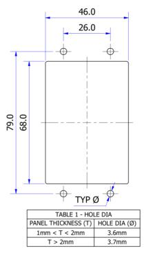
Panel cut-out to flush mount relay for use with rear connect TBD-R2 base
