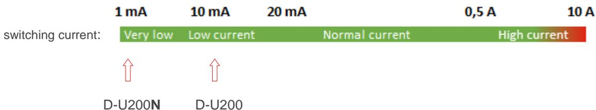
Advise to always use gold plated contacts when switching very low currents to prevent contact corrosion (D-U200N-E).
