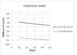
By connecting 2 contacts in series the DC current breaking capacity is increased by 50 %. Electrical lifetime is tested under laboratory conditions with switching frequency 0.33 Hz.
