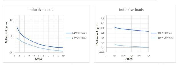
By connecting 2 contacts in series the DC current breaking capacity is increased by 50 %. Electrical lifetime is tested under laboratory conditions with switching frequency 0.33 Hz.
