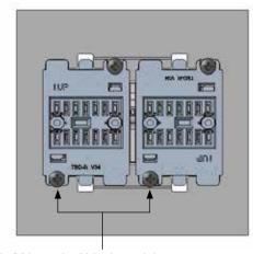
4x M4 terminal block retaining screw
