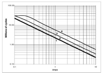
By connecting 2 contacts in series, the DC current breaking capacity is increased by 50%. In all the cases, these relays guarantee a right performance during 50,000 operations.
