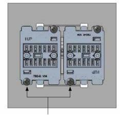
4x M4 terminal block retaining screw
