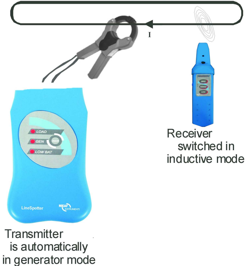
Fig. 8. Injection of test current into closed tested loop by means of current clamp
