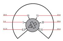
Example: if the set current is 10 A and the time delay is 5 seconds, the relay will switch when the current exceeds the set value of 10 A for minimal 5 seconds
