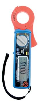
At first, the NI 333 looks like a normal current clamp. Nevertheless, the special integrated technique of the jaw enables the user to measure very low or differential currents. The NI 333 is designed with an ergonomic housing with a wide jaw (opening). With this jaw, conductors up to 30 mm can be measured easily.
