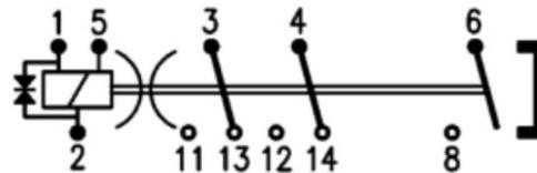
Remark: diagram shown is DC version with delay-on and delay-off both adjustable.
