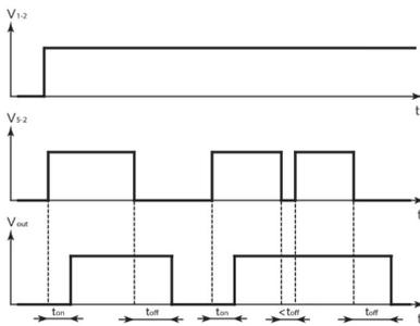
If the time between a falling edge and a rising edge of the command signal is less than the delay (toff) the relay will remain energized.
