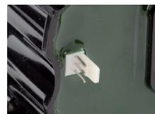
Molex output connector for MSA sensors
