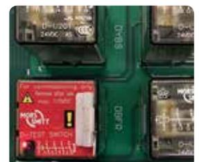
Test system by simulating energized relay: Contacts are manually switched
