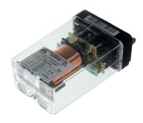
The N.S1-R-24-4.0.4 is a 24 VDC track side safety relay for the signalling railway market. It is a single module plug-in relay with positive mechanical keying, equipped with 4 heavy duty normally open contacts and 4 normally closed contacts.
