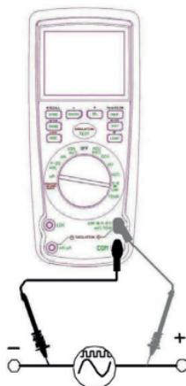
1. Set the rotary function switch to the green Hz/% position
