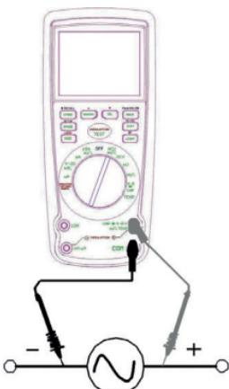
1. Set the functionswitch to the green VAC/Hz/% position
