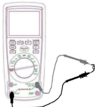
1. Set the rotary function switch to the INSULATION position and press the RANGE button to select the voltage which displays on the top left corner
